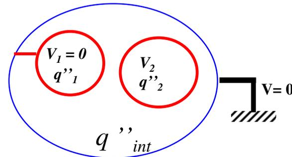
$$q''_1 = C_{12} V_2 \quad q''_2 = C_{22} V_2$$
