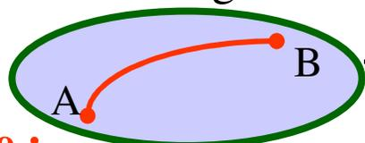
$$-\int_A^B \vec{E} \cdot d\vec{L} = V(B) - V(A) = 0 \quad \text{car } E = 0$$
