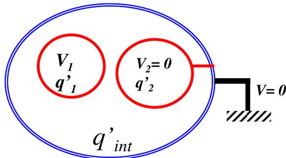
$$q'_1 = C_{11} V_1 \quad q'_2 = C_{21} V_1$$
