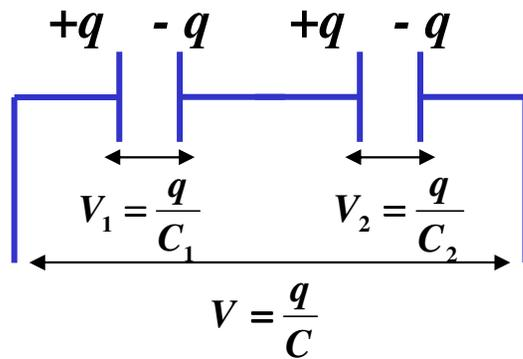
$$V = V_1 + V_2$$
